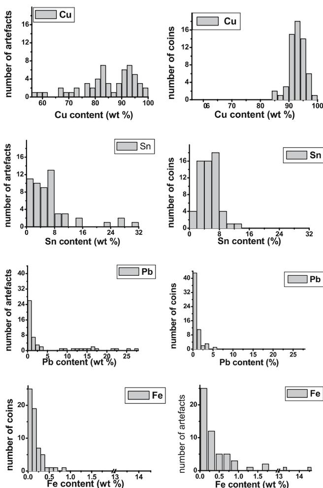
**FIGURE 2** Frequency distribution of Cu, Sn, Pb and Fe content for the selected bronze artefacts found in different archaeological areas of the Mediterranean basin and for a nearly equivalent number of bronze Punic Coins of the same series, found together in the same archaeological excavation in Sardinia (Italy), *left and right* column, respectively
