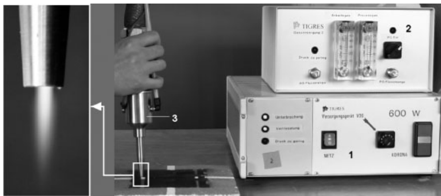
Figure 1. Plasma source: "Plasma-BLASTER MEF"; 1, power supply unit; 2, gas supply; 3, treatment head.
