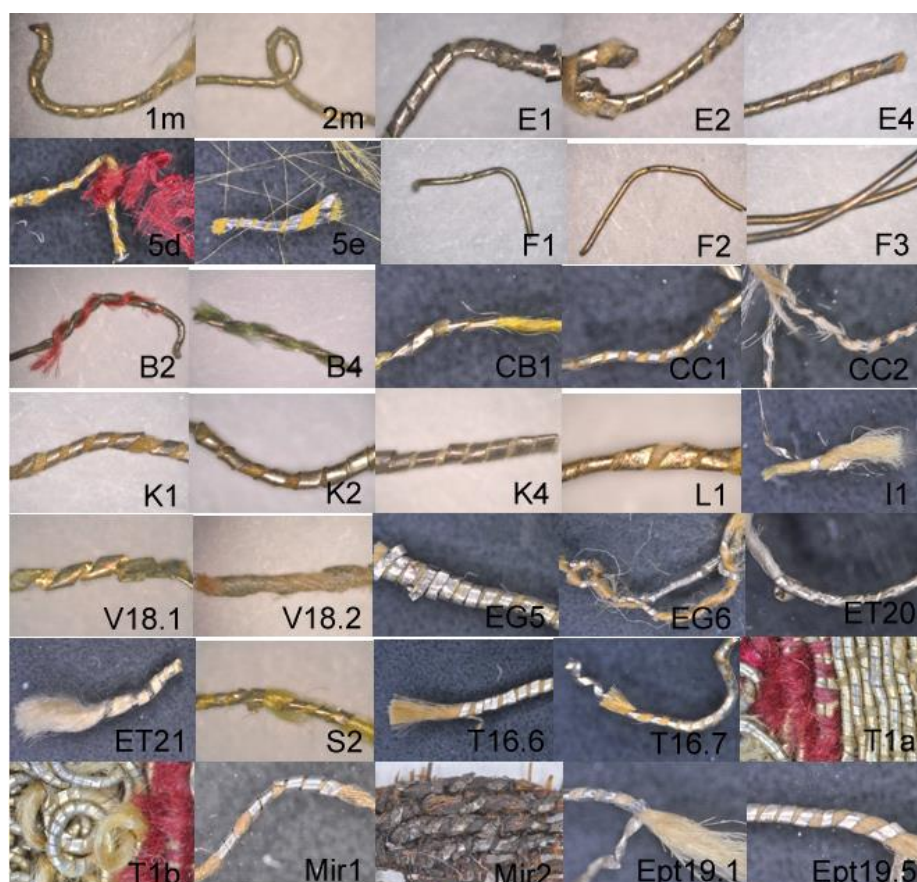
Fig. 1. Metal threads analyzed by \mu ATR and ATR spectroscopy
