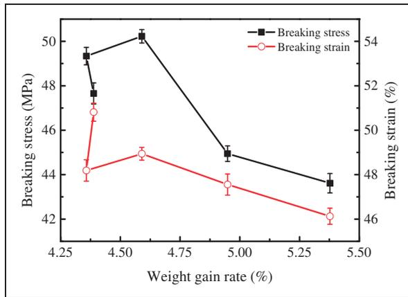
**Figure 7.** Breaking stress and strain change with weight gain rate of the fabrics.
