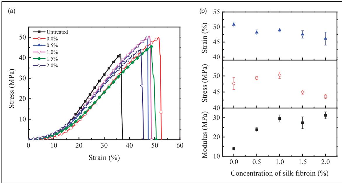
**Figure 6.** (a) Stress–strain curves and (b) mechanical properties of the silk fabrics treated by transglutaminase + sodium caseinate and sprayed with silk fibroin with different concentrations.
