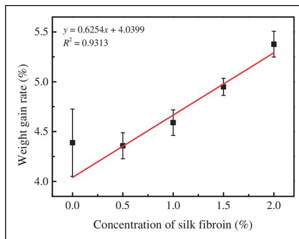
**Figure 5.** The weight gain rate of fabrics with the concentration of silk fibroin.
