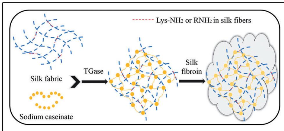
**Figure 2.** Schematic diagram of the sample preparation process. TGase: transglutaminase.
