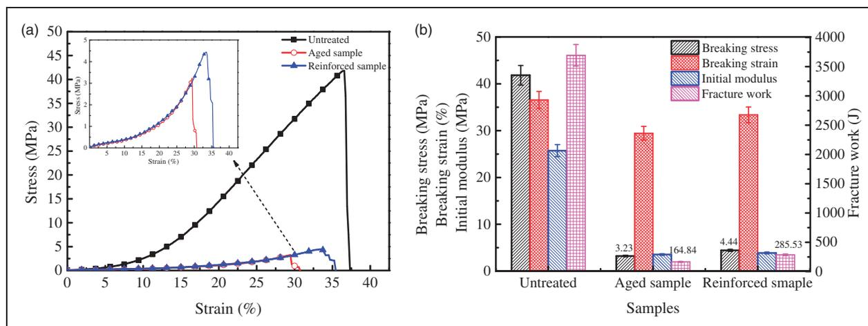
Figure 11. Alkaline aging and reinforcement samples: (a) stress–strain curve; (b) mechanical properties.
