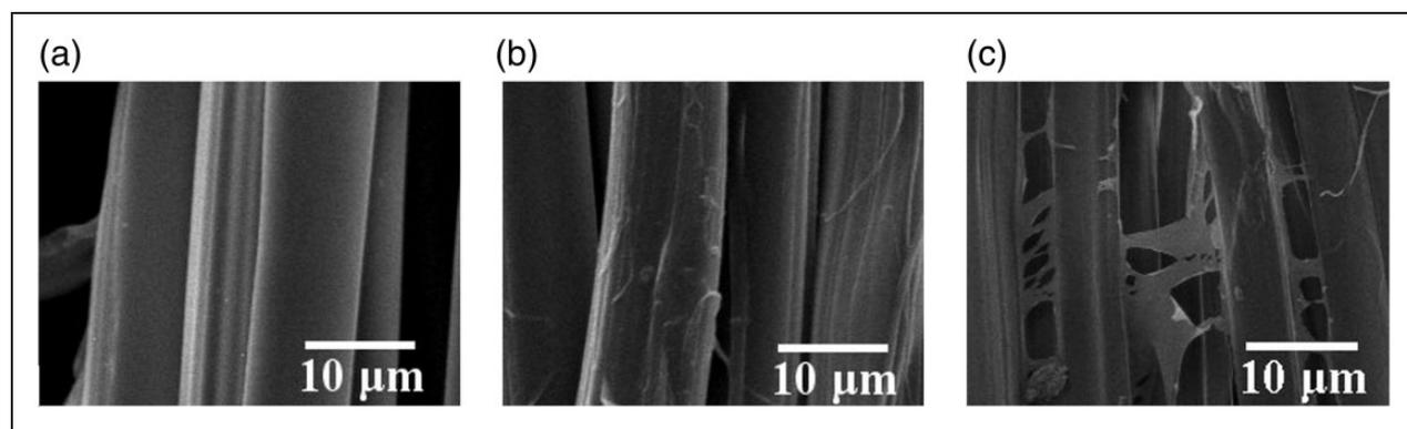
**Figure 9.** Scanning electron microscopy images of silk fabric: (a) untreated; (b) transglutaminase (TGase) + sodium caseinate (SC) treated; (c) TG + SC + silk fibroin treated.
