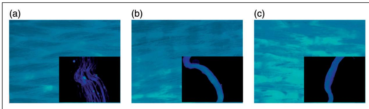
**Figure 8.** Photograph of silk fabric under the ultraviolet light of a fluorescence microscope: (a) untreated; (b) transglutaminase (TGase) + sodium caseinate (SC); (c) TGase + SC + 1.0% silk fibroin.
