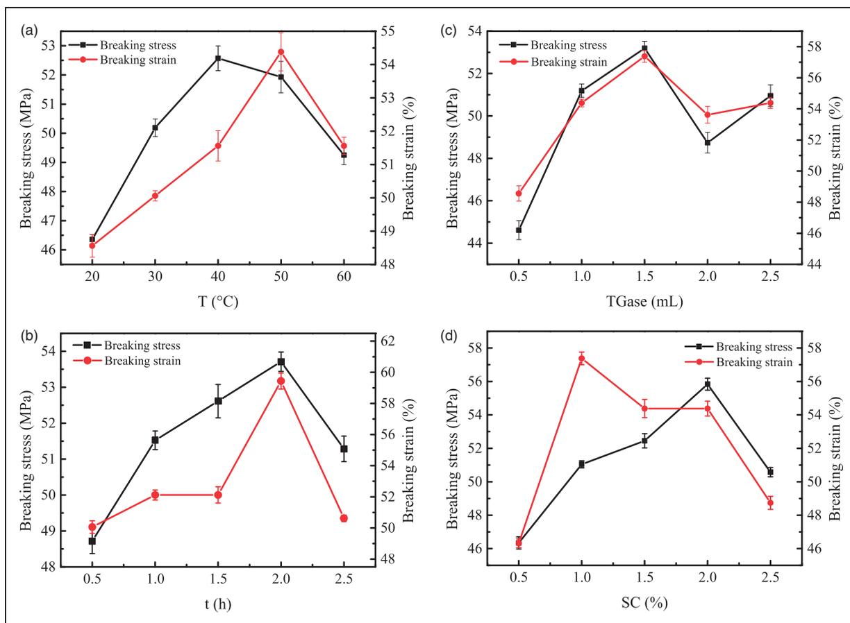
**Figure 3.** The changes of breaking stress and strain of transglutaminase (TGase) + sodium caseinate (SC) samples with (a) temperature  $T$  ( $^{\circ}\text{C}$ ), (b) time  $t$  (h), (c) TGase (mL), and (d) SC (%).
