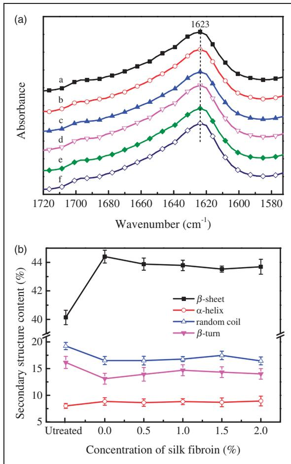
**Figure 10.** (a) Fourier transform infrared spectra and (b) the fitting results of the secondary structure of silk fibers treated with different concentrations of silk fibroin (SF). (Samples: a: untreated; b: transglutaminase (TGase) + sodium caseinate (SC); c: 0.5% SF + TG + SC; d: 1% SF + TG + SC; e: 1.5% SF + TG + SC; f: 2% SF + TG + SC.)
