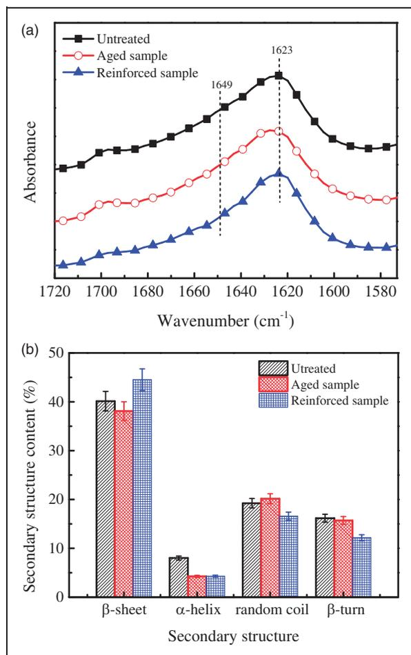
**Figure 13.** Alkaline aging and reinforcement samples: (a) infra-red spectrum; (b) secondary structure content.
