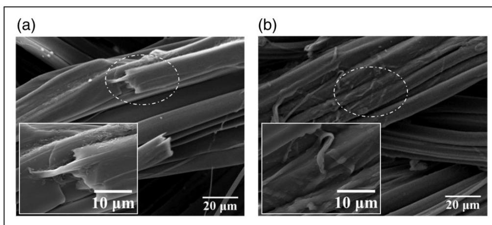
Figure 12. Scanning electron microscopy images: (a) alkali aging sample; (b) alkali aging reinforcement sample.
