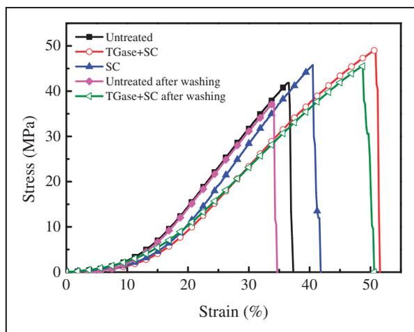
**Figure 4.** Under the optimal conditions (50°C, 2 h, 1.5 mL transglutaminase (TGase), 2% sodium caseinate (SC)), the stress-strain curve of the fabric.
