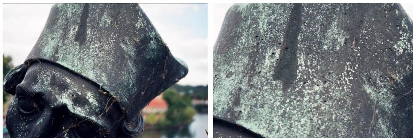
Figure 9. Detail of bronze surface with open holes.
