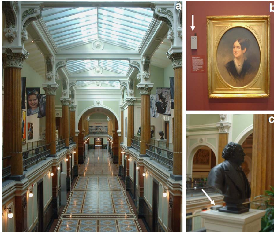
Fig. 4. (a) the Great Hall viewed from the third floor mezzanine showing skylights on the south wing of the building; (b) light monitor E112.EFW vertically installed near an oil painting; (c) light monitor S321.H horizontally installed on a sculpture pedestal. (Photos: Julio M. del Hoyo-Meléndez).
