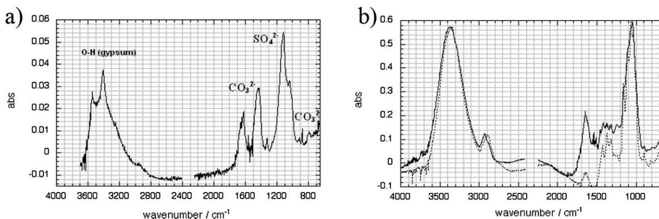
**Fig. 3** (a) Infrared spectrum of soil particles where gypsum ( $\text{CaSO}_4 \cdot 2\text{H}_2\text{O}$ ) and calcium carbonate are present; (b) representative infrared spectra for the whitish crust (full line) compares well with the spectra obtained for the paper used for storage protection (dotted line).
