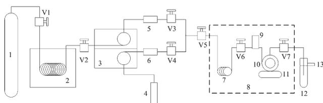
**Fig. 4** Experimental cleaning apparatus: (1)  $\text{CO}_2$  cylinder; (2) refrigeration unit; (3) high-pressure liquid pump, master and slave Gilson pumps; (4) co-solvent; (5) and (6) check-valves; (7) pre-heater; (8) thermostated bath; (9) pressure transducer; (10) high-pressure visual cell; (11) cell support; (12) trap; (13) vent; (V1) to (V7) high-pressure valves.
