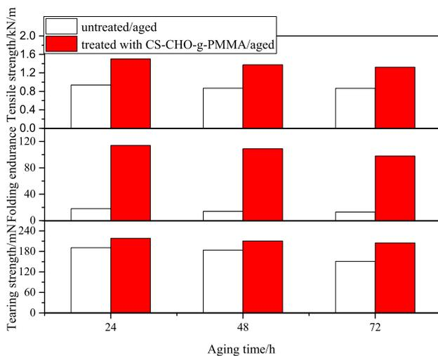
**Figure 3:** Effect of the aging time on the mechanical properties of paper.
