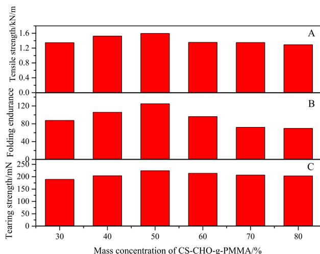
**Figure 1:** Effect of the concentrations of CS-CHO-g-PMMA on the tensile strength (A), folding endurance (B), and tearing strength (C) of paper.
