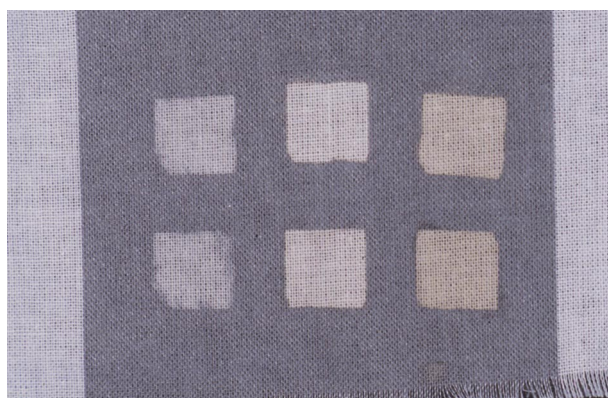
Figure 3. Laser test cleans on artificially soiled new cotton. The test areas are approximately 1.5 cm \times 1.5 cm. Upper row (left to right): 1) 266 nm, 0.15 J/cm 2 ; 2) 532 nm, 3.2 J/cm 2 ; 3) 1 064 nm, 2.7 J/cm 2 . Lower row (left to right): 1) 266 nm, 0.1 J/cm 2 ; 2) 532 nm, 1.1 J/cm 2 ; 3) 1 064 nm, 1.0 J/cm 2 .
